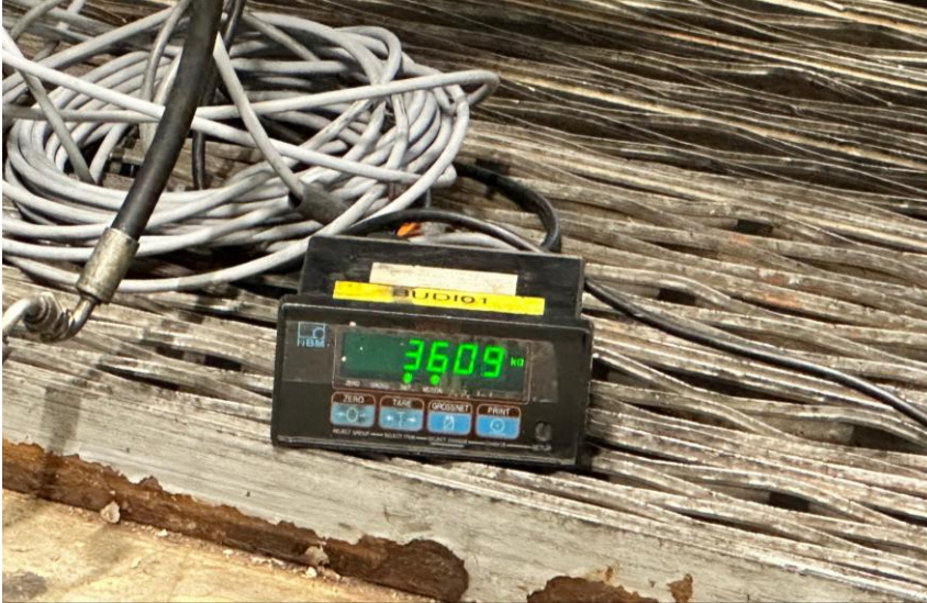
Photo 3. Three-point bending force was measured 3609KG (35.4kN)
