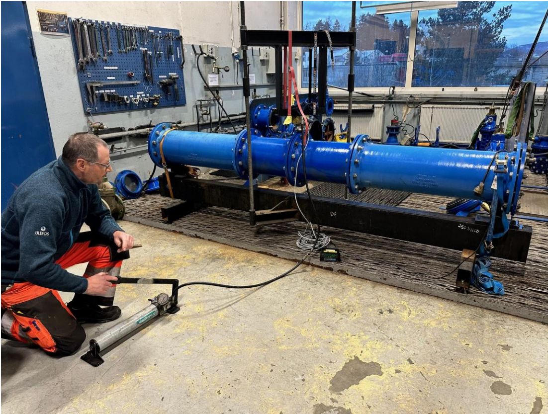
Photo 1. Test setup. 3-point bending test is performed.
